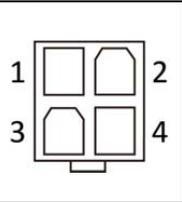
**DC\_JACK:** DC input connector (+9V~24V)
