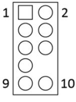
**AMP1: 4ohm 3Watt Amplifier output pin header**
